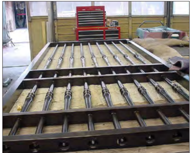
Figure VI-12. Oil-rubbed bronze gates prepared for installation at the State Capital in Harrisburg, Pennsylvania.
