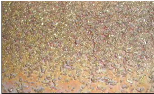
Figure VI-2. As natural a look as you can get: unfinished copper cathode, 99.9% pure. Typically shipped as melting stock to mills or foundries, cathodes may also be cast into wire rod, billets, cakes or ingots and alloyed with other metals.
