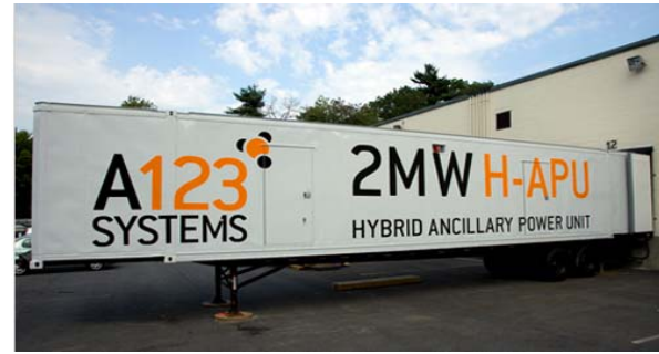
Figure C-1. Xtreme Power 1.5 MW Lead-Acid Battery System and A-123 2 MW, 500 kWh Li-Ion System
