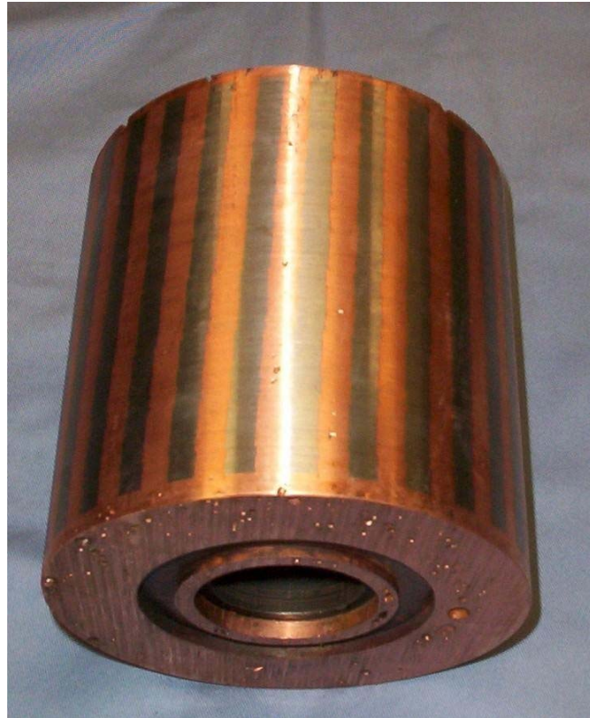
Figure 12 – Photograph of copper rotor turned on the OD to expose the conductor bars. Trapped air bubbles are not seen in the bars but are clearly visible in the end ring.
