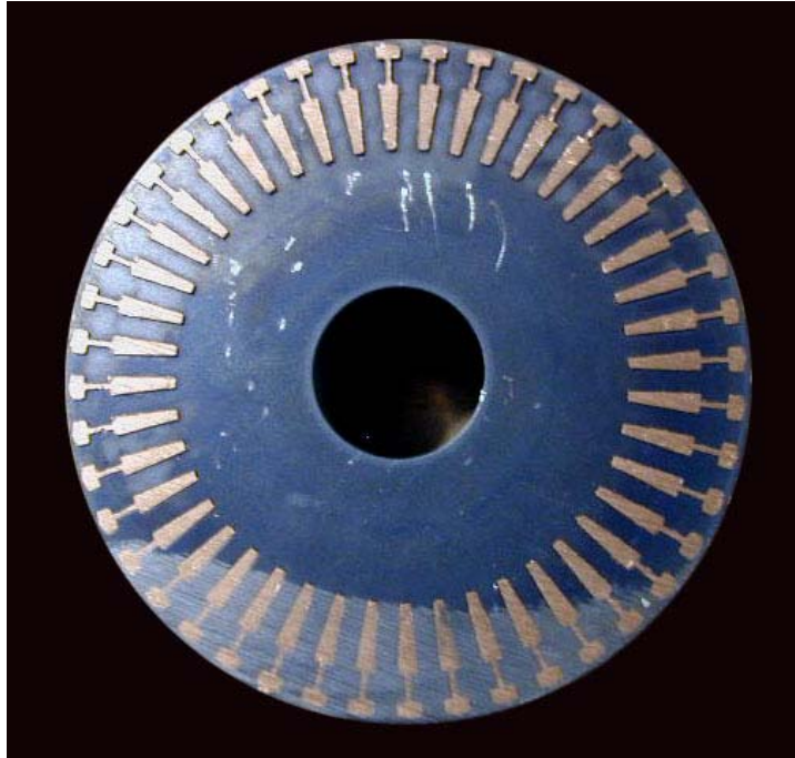
Figure 16 - Cross-section of a die cast copper rotor showing complete filling of the conductor bars.
