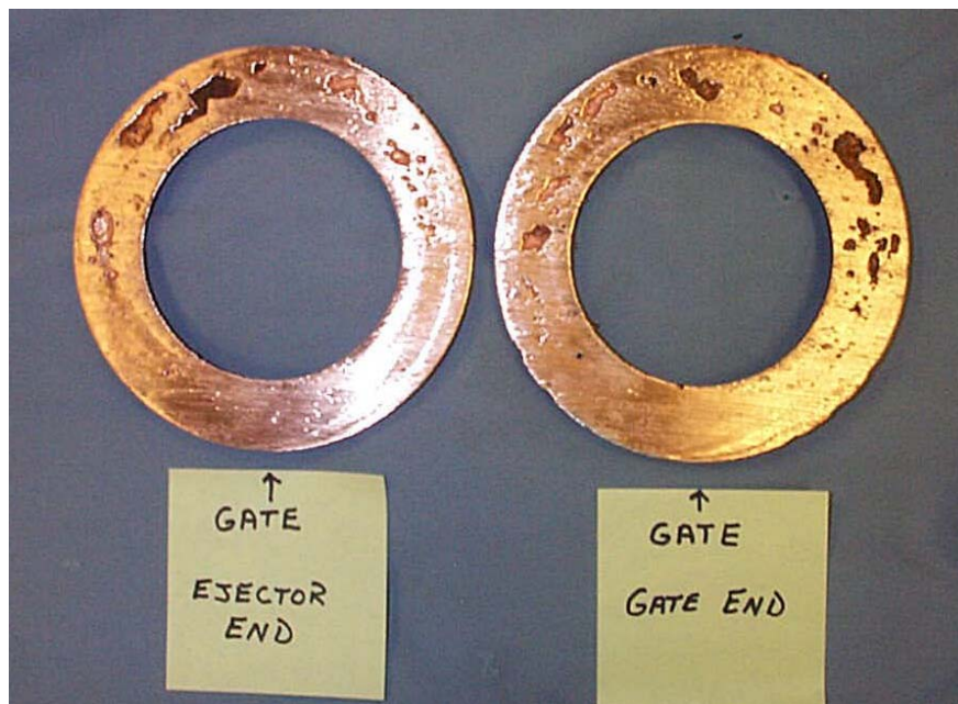
Figure 9 – Photographs of sectioned end rings from a 15 Hp (11.2 kW) copper rotor typical of baseline die casting conditions.
