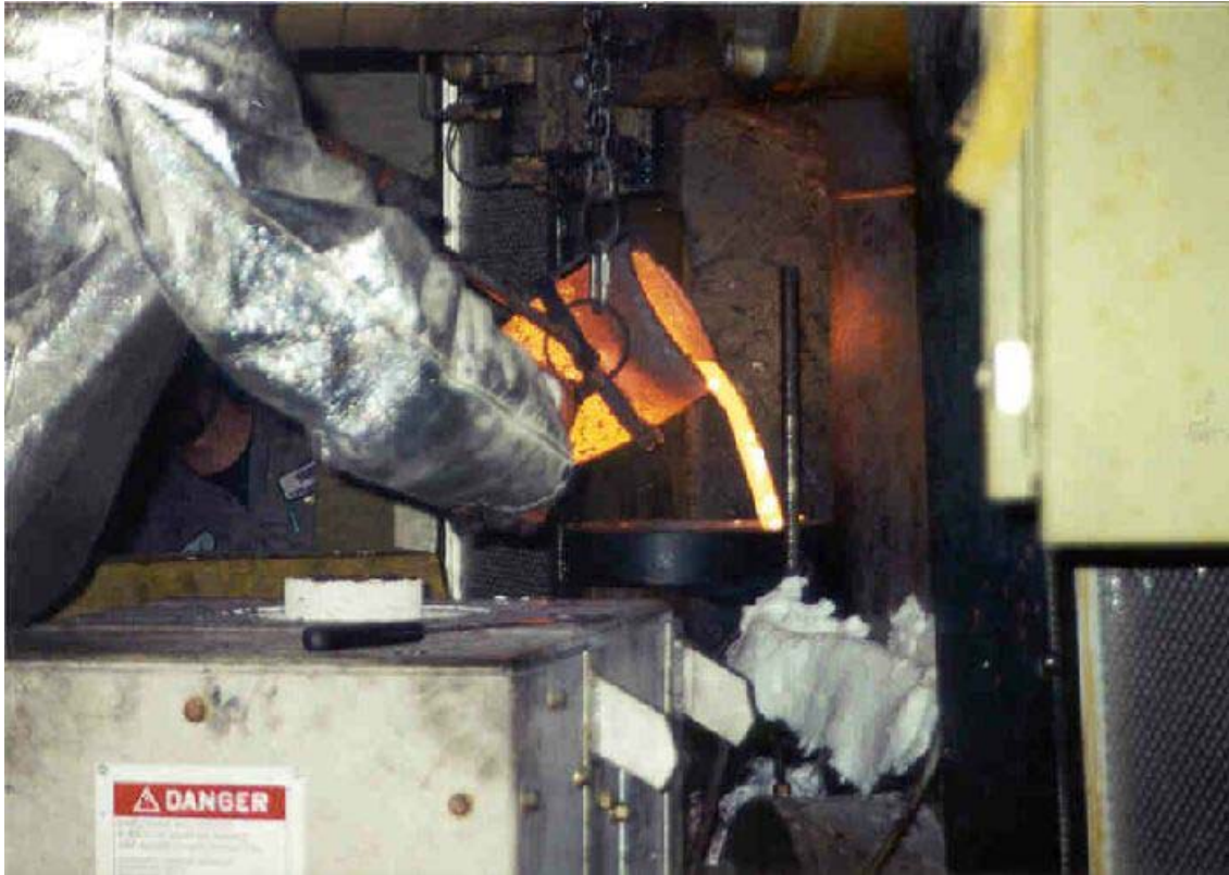
Figure 27 - Transfer of single shot of molten copper from double coil induction melting unit to shot sleeve in the CDA development work at Formcast.
