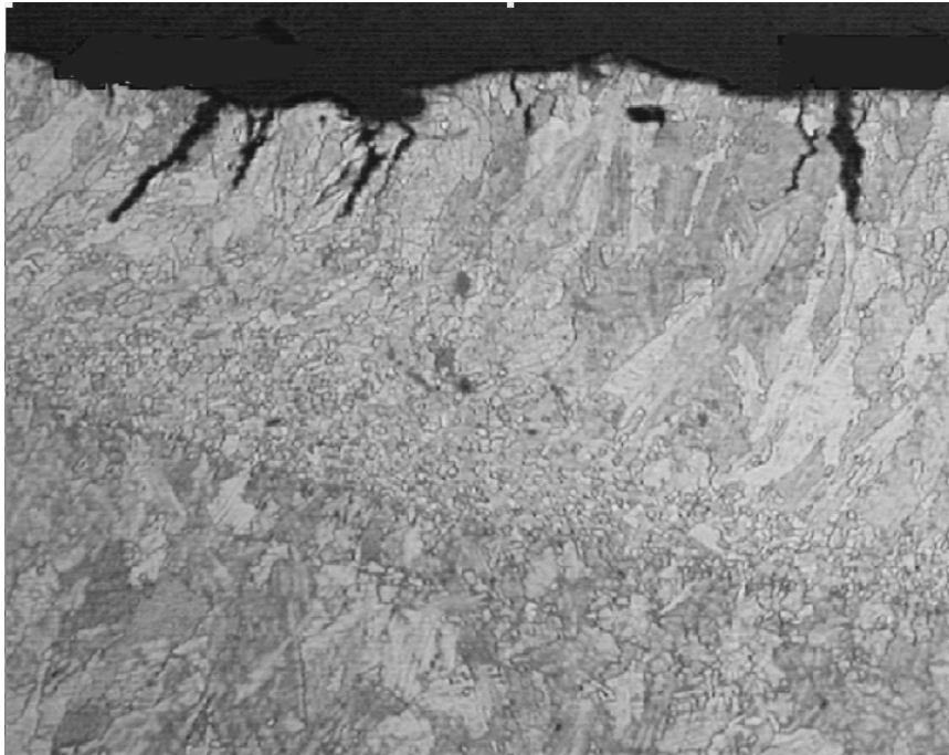
Figure 14 - Macrostructure of cast copper showing dendritic grain structure at the steel chill interface and a largely coarse equiaxed structure in the center. Very small volume fractions of oxide and porosity are seen. 50X.
