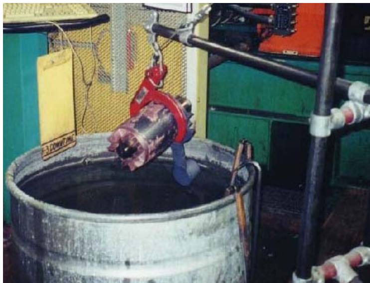
Figure 8 - Water quenching of die cast copper rotors after extraction from dies. This operation reduces cooling time and although not necessary for performance, is an aid to productivity by shortening handling time. Operation could be mechanized for production.
